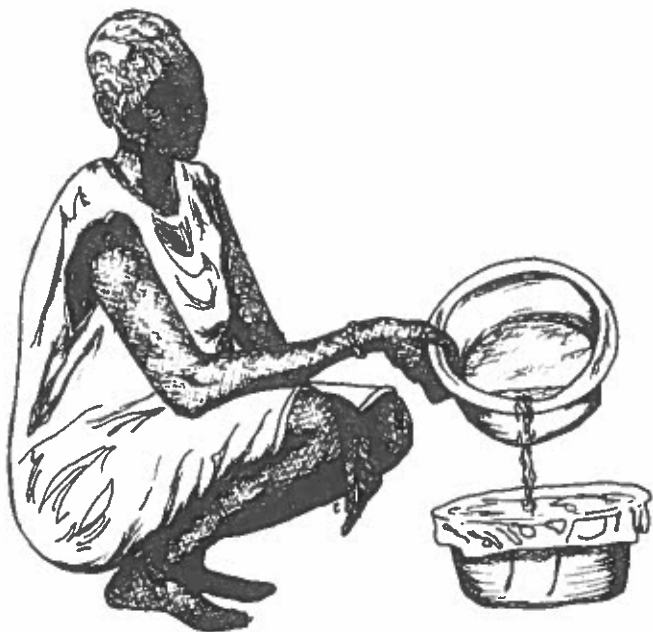
Figure 18-9. Filtration Through Overlaid Layers of Fabric Cloth or Nylon Mesh Filters Can Remove Larger Particles.
